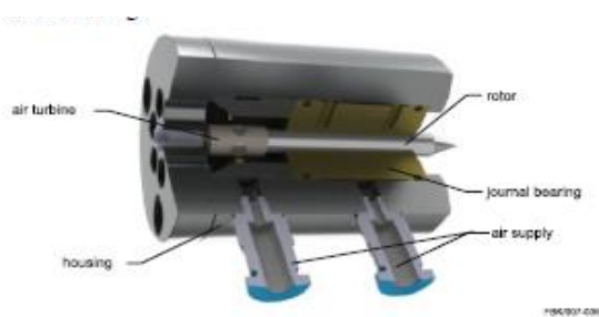
Fig:1 DESIGN OF A COMPACT AIR BEARING SPINDLE
