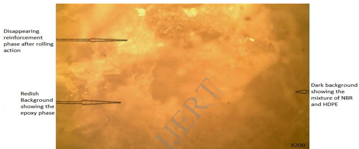
Plate 3: Micrograph showing the disappearing reinforcement phase after rolling, reddish background showing the epoxy phase and dark background in the presence of NBR and HDPE mixture (X200)
