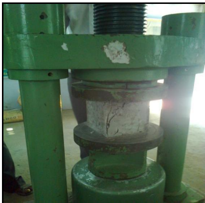
Fig. 1. Determination of compressive strength of cube
