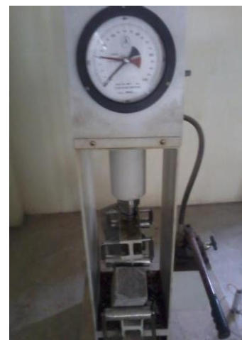
Fig.3. Determination of Flexural Strength of Prism
