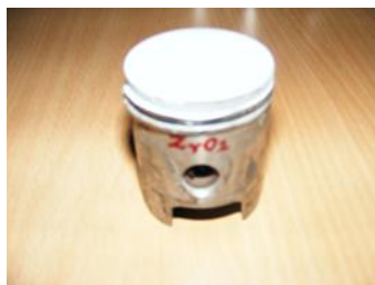
Fig.2: Zirconium Dioxide Coated Piston
