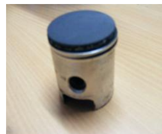
Fig.3: Titanium Dioxide Coated Piston
