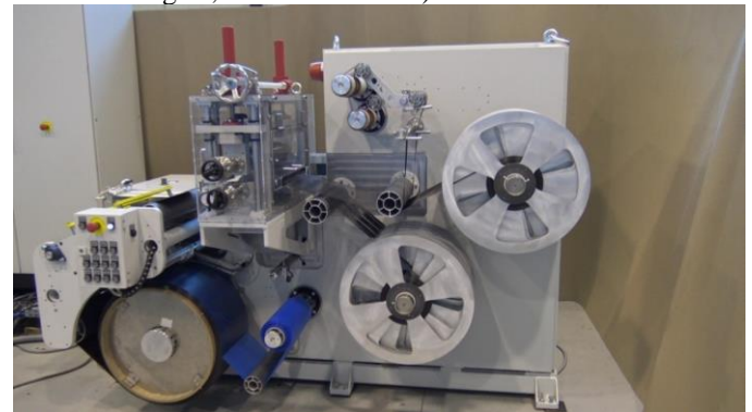
Fig. 1 Machine for shear slitting of UD prepreg tapes (Mikrosam D.O.O.)
