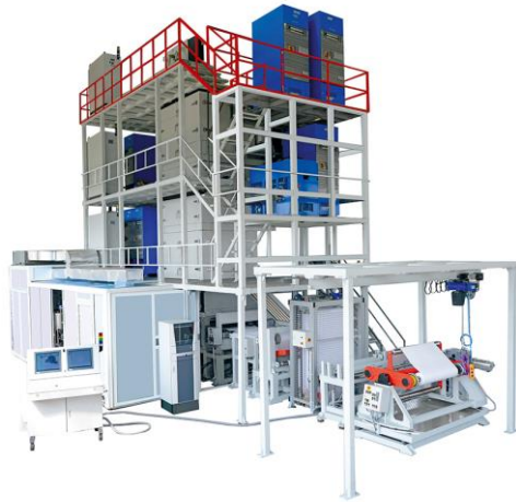
Fig. 1 Vertical impregnation lines.
