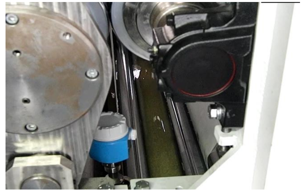
b) Resin with deep impregnation resin and dosing rollers
