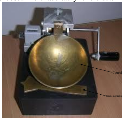
Fig. 2. Equipment for determining the liquid limit in the laboratory
