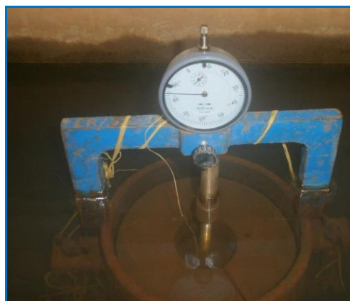
Fig. 4. Linear swelling measurement device on a CBR mold in the laboratory
