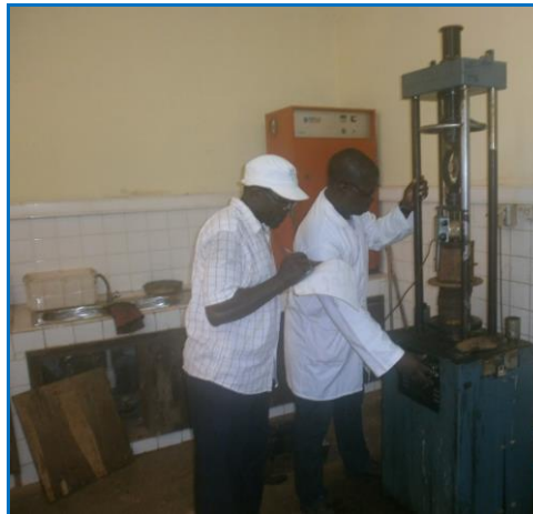
Fig. 3. Punching a CBR specimen in the laboratory
