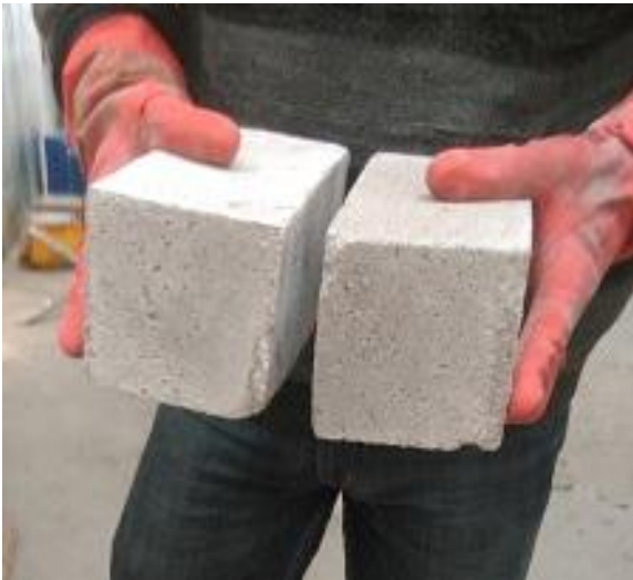
Fig. 8. Striking bricks for soundness test
