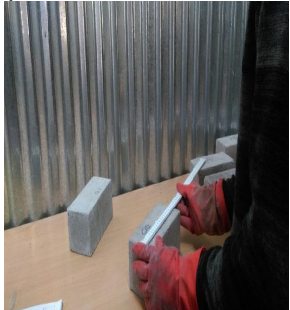
Fig. 9. Determination of shape and size
