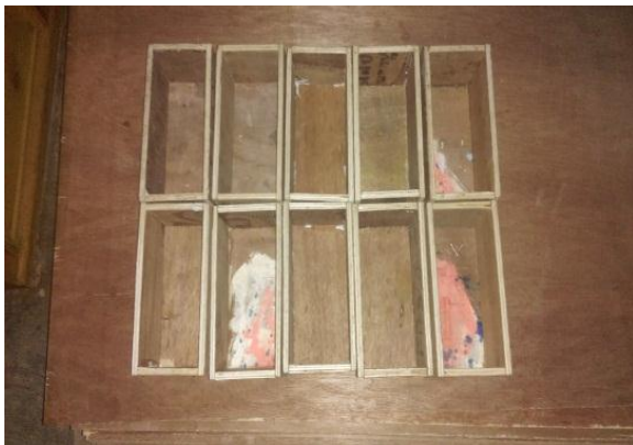
Fig. 3. Moulds for manufacturing bricks
