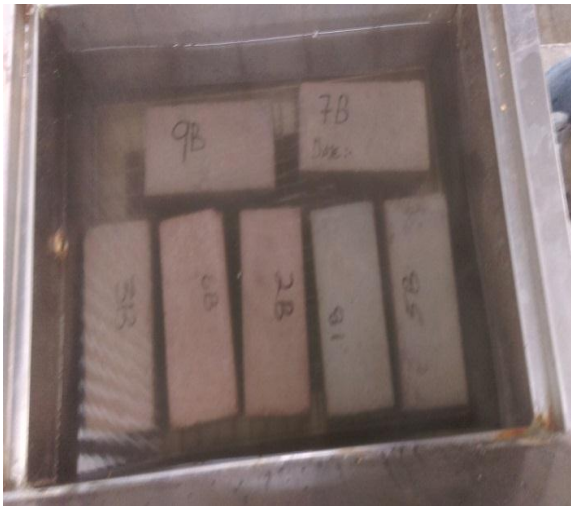
Fig. 5. Brick samples in water for water absorption test
