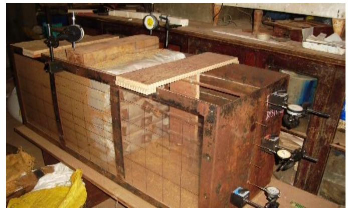
Fig.2.3. View of the model nailed wall
