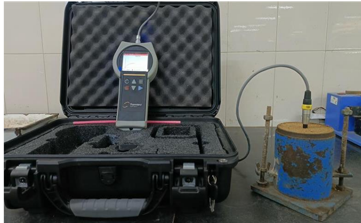
Fig. 3 Conducting Test in a Compacted Soil Mould
