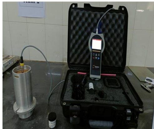
Fig. 5 Representative Experimental Setup for Thermal Resistivity Testing across Varying Moisture Contents
