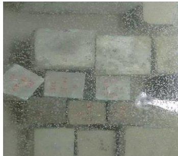
Figure 8: Externally Self cured concrete specimens
