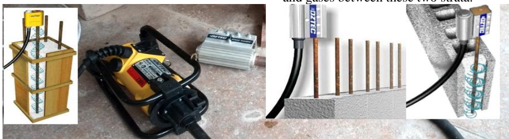
Figure 1: Oztec's rebar shaker (Courtesy Oztec 2012)
