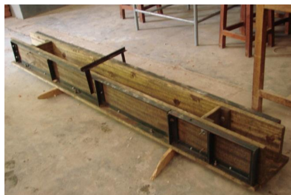
Fig. 3.15 Mould for Beam Specimen
