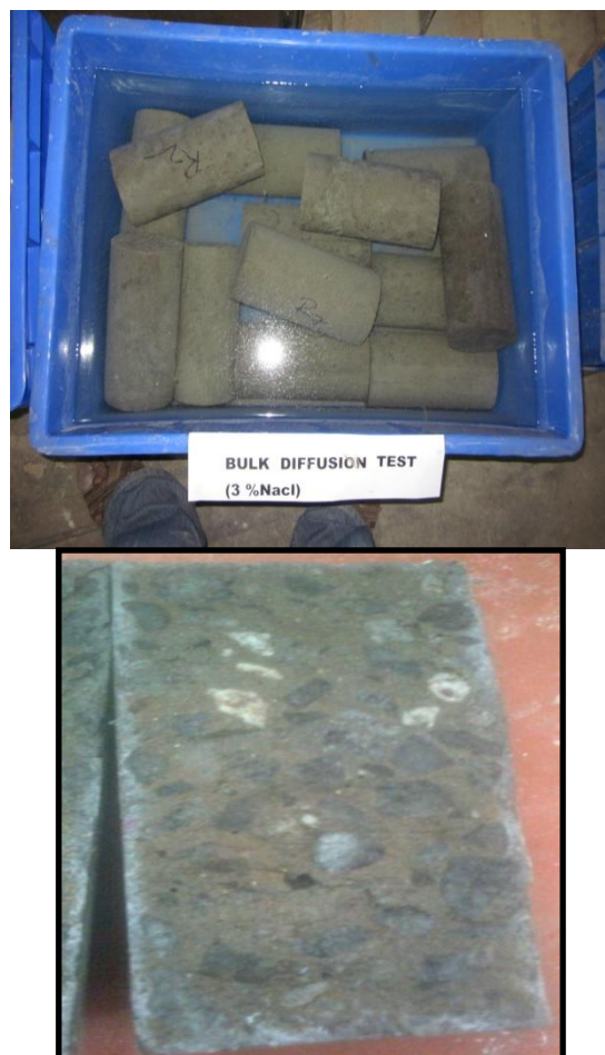
Fig 4.16 Depth of penetration of chloride ions
