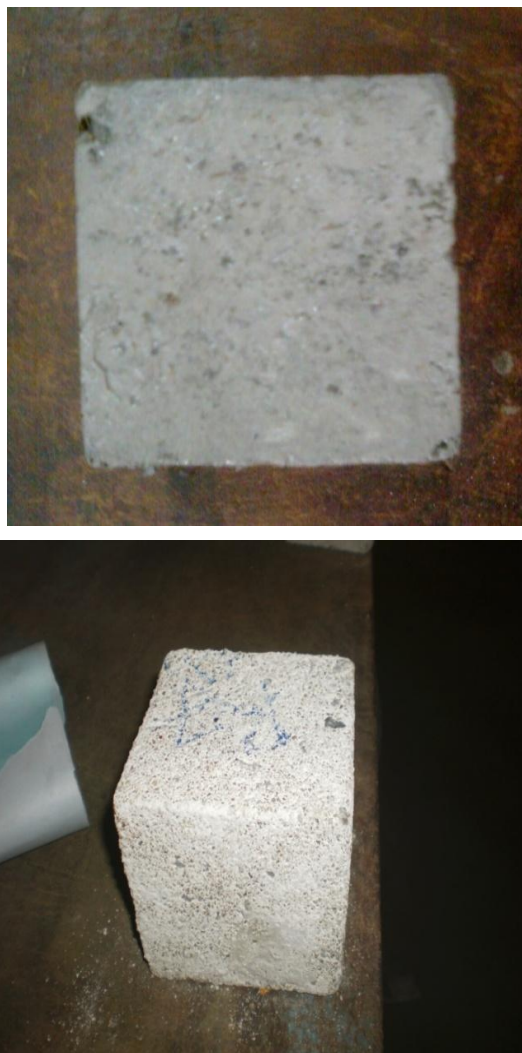
Fig 4.11 Appearance of concrete cube before and after acid exposure
