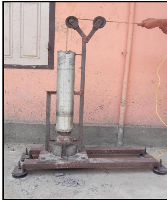
Fig.3.8 Test equipment for impact strength test
