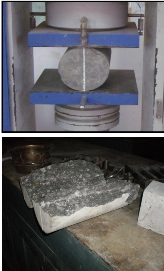
Fig 3.4 Split tensile strength test on cylinder
