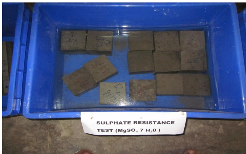
Fig 3.10 Specimens exposed to sulphate solution
