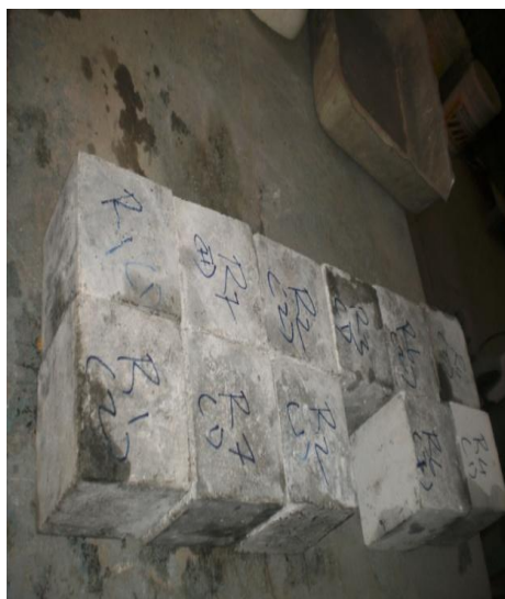
Fig 4.14 Appearance of cube after sulphate exposure
