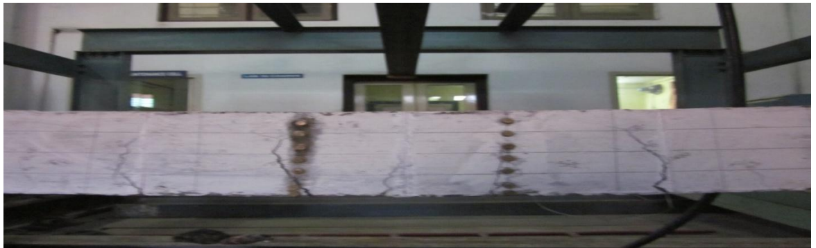
Fig. 4.36 Crack Pattern of R 5 Beam under Flexure
