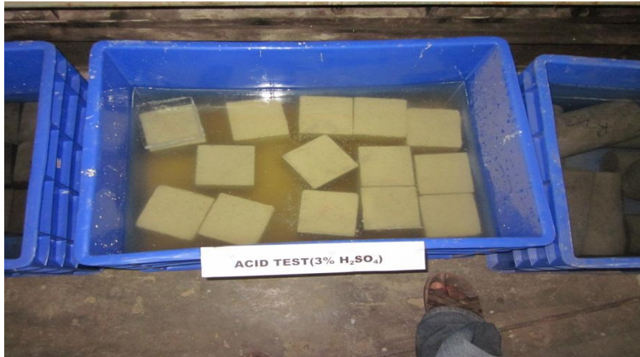
Fig 3.9 Specimens exposed to 3% sulphuric acid solution
