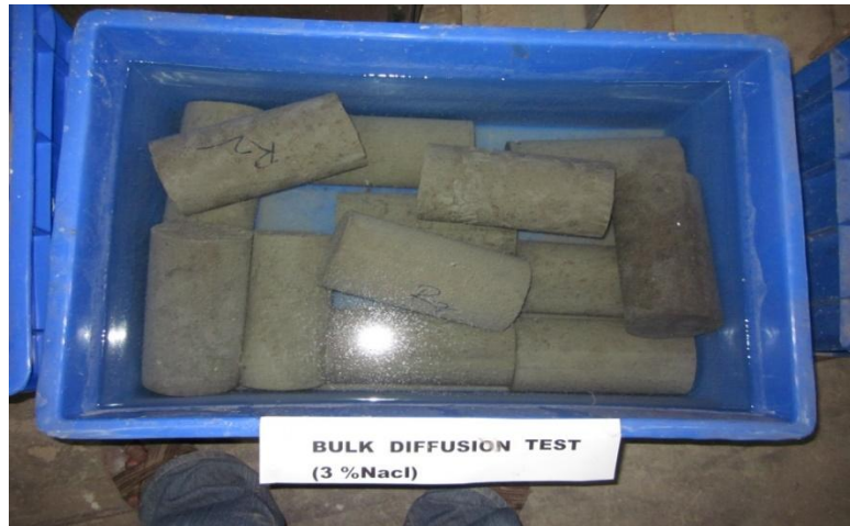
Fig 3.11 Specimens exposed to NaCl solution
