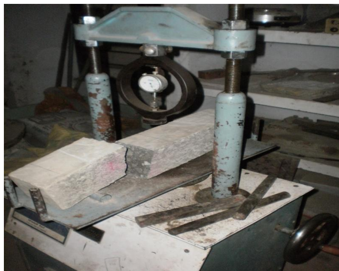
Fig 3.6 Flexural strength test on beam before and after loading
