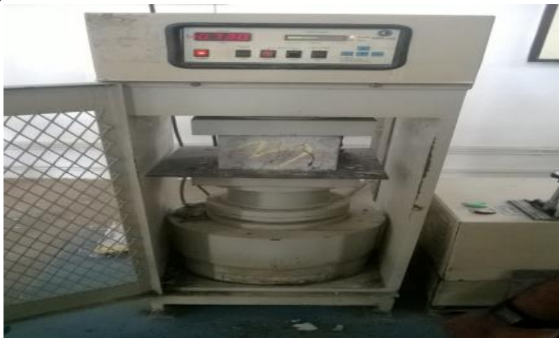
Fig 2.1 Compression test for cube specimen
