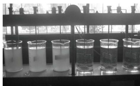
Figure - 2 Conventional jar test apparatus
