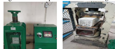
Fig-6: Compressive & Flexural strength test.
