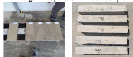
Fig-5: Beam samples for flexural strength
