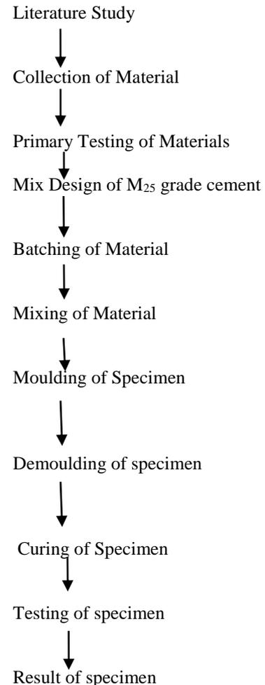
Fig 1: This is the schematic representation of our project
