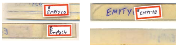
Fig. 1. Epoxy/Ca 2 SiO 4 Composite Test Coupons
