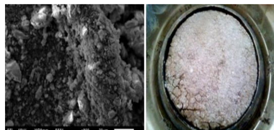
Fig 4 shows Sem and snap shot image of treated expansive clay with aquaculture sludge
