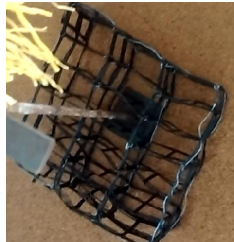
Fig 2. Placing anchor plate and geocell at required embedment depth
