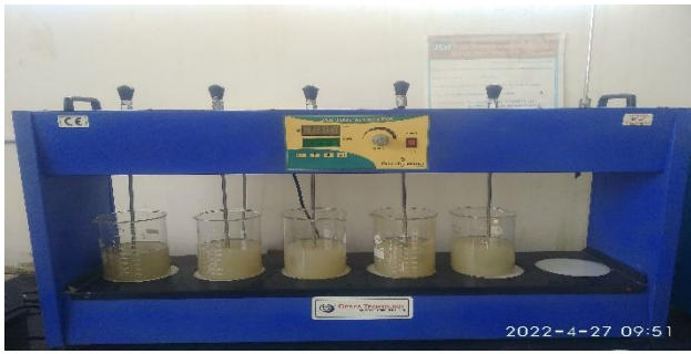
Fig 4 Standard jar test
