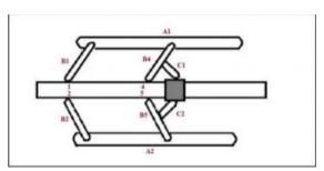
Operate the motor wheel the robot remote is connected. The camera is connected to the display equipment(output) via long cable wound upon a winch There are 6 wheels the dia. Of wheel 72mm. There are 6 D.C motor having 10rpm & 12v.There are 2 BO motor having 60rpm & 3-9v.The BO motor is used for actuate the camera & light and it is fixed to the front side of the robot. The spring is attached to
