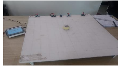
Fig 12: Condition of object placed equidistant from sensors
