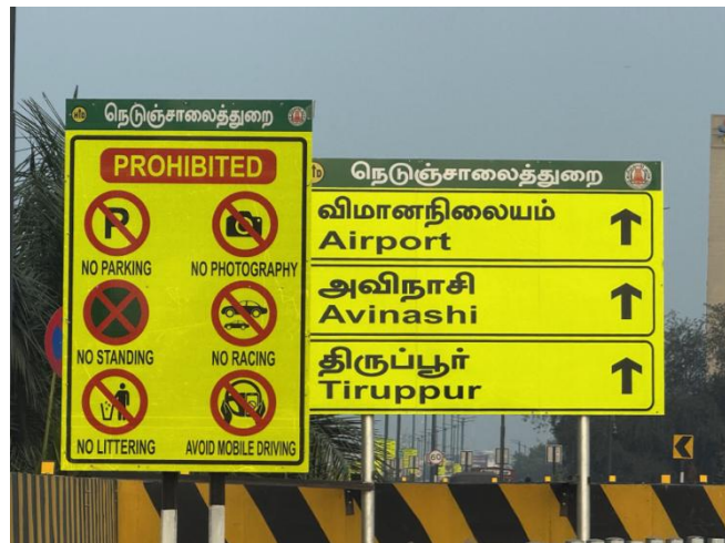
Fig 29. Retro Reflective Boards
