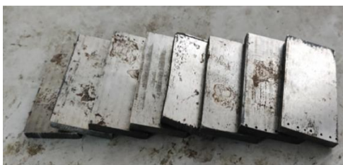
Figure 2. Specimen after surface grinding
