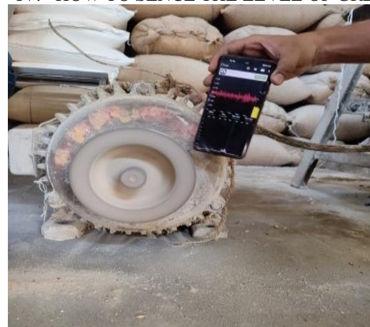
Figure 3: More distortion at low greasing level
