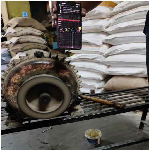
Figure 4: less distortion at high greasing level
