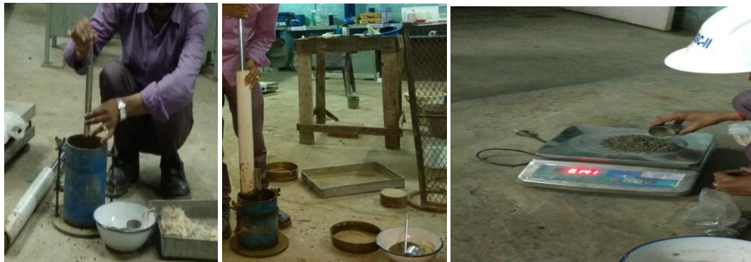
Figure 4 Process of preparation of stone column by clay soil, jute geotextile and stone chips
