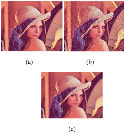
Fig. 8 Execution of PRNM filter - Removal of impulse noise from lena colour 8(a) Original image 8(b) noisy image 8(c) Denoised image
