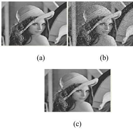
Fig. 7 Execution of PRNM filter - Removal of impulse noise from lena gray 7(a) Original image 7(b) noisy image 7(c) Denoised image
