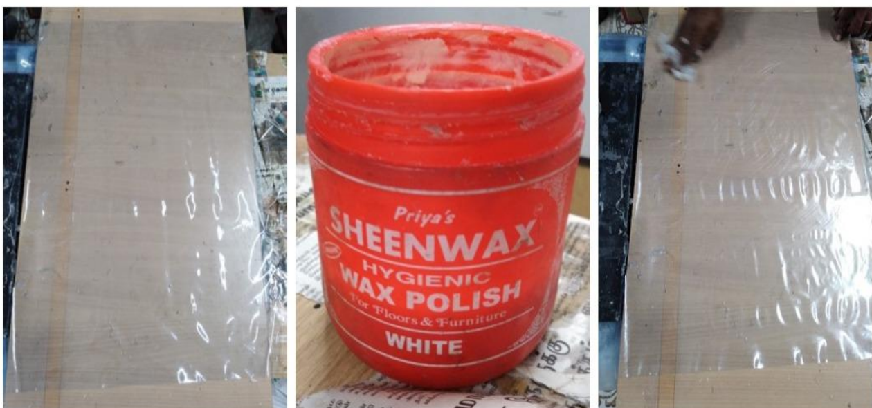
Figure-5: Flat hard board with plastic sheets, release gel and release gel coating on moulding surface
