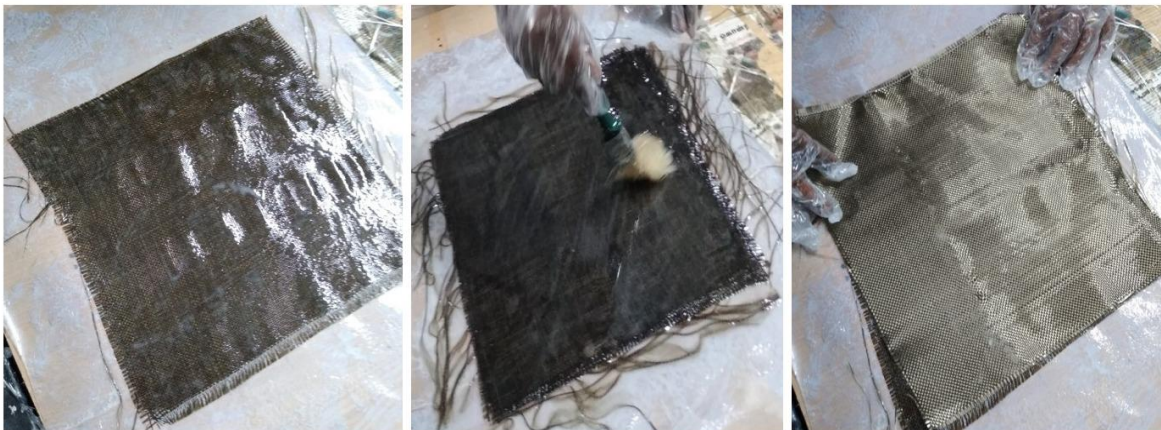
Figure-7: Layer by layer preparation of laminate through impregnation of resin with brush
