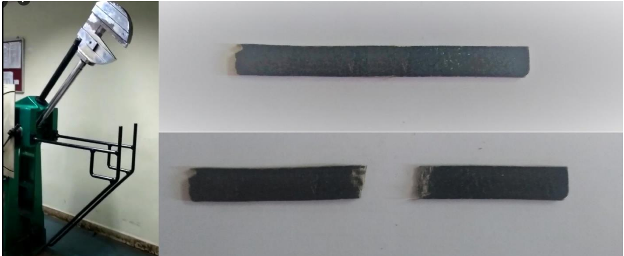
Figure-12: Charpy impact test machine, specimens before and after impact test
