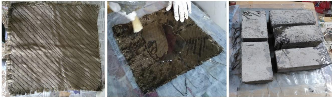
Figure-8: Impregnation of resin into stitched plies and application of uniform load over it
