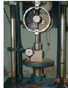
PLATE 3 VIEW OF FLY ASH BLOCK COMPRESSIVE TESTING
