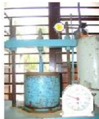
Plates 4 Consolidation Test Arrangement
