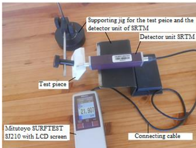
Fig. 3: Surface finish measurement setup with Mitutoyo SURFTEST SJ-210
