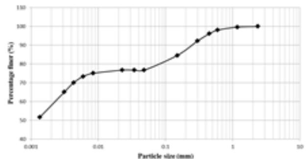
Fig. 1. Particle size distribution of natural soil.
