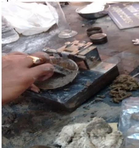
Figure 5: Casagrande apparatus for determination of consistency limit.
