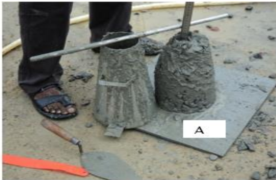
Plate 1: A: slump test showing true slump; B: slump test showing shear slump
