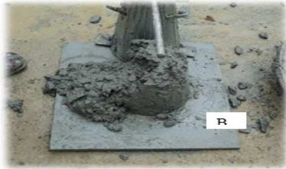
Plate 1: A: slump test showing true slump; B: slump test showing shear slump
