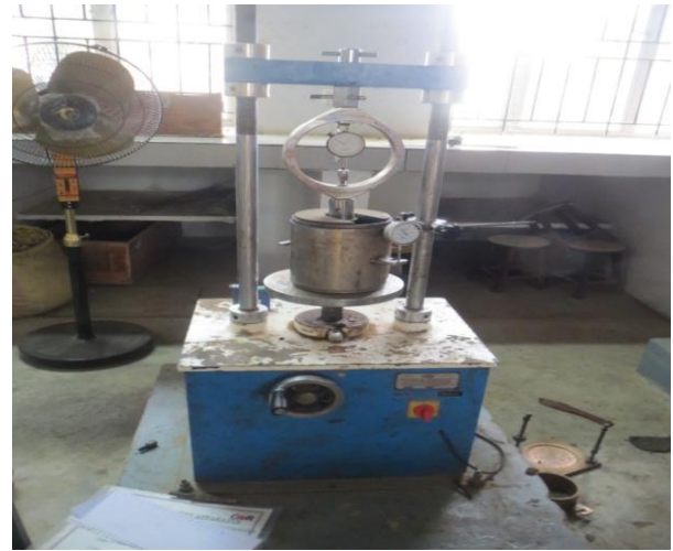
Fig.2 Test setup to find CBR value of soil and Aggregate
