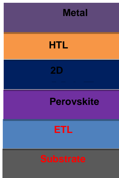
Fig.1.Schematic diagram of 2D-MOF Perovskite thin film.
