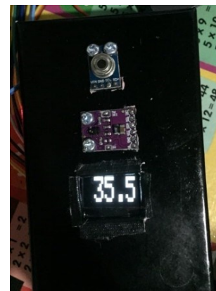
Fig. 16. Temperature data display on OLED display
