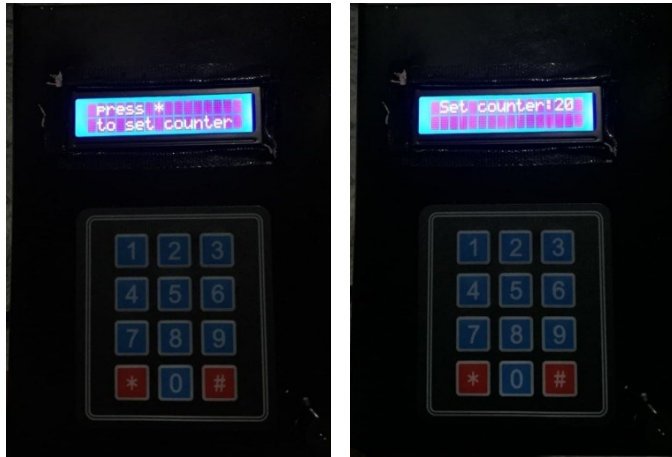
Fig. 14. Entering user input to set the counter
