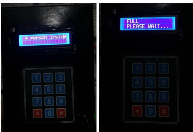
Fig. 15. Displaying customer occupancy on LCD display
