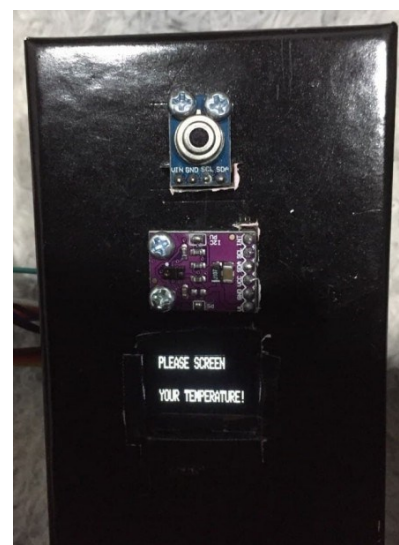
Fig. 17. Text display when temperature exceed 37.5 °C
