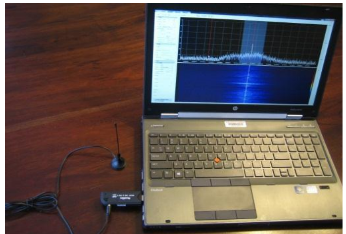
Fig.5. The RTL-SDR Based WBFM Receiver Setup
