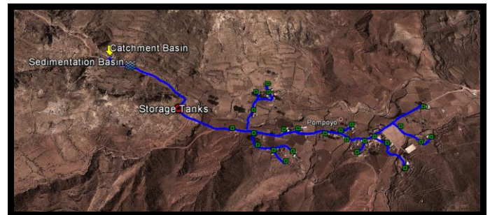
Figure 1. Schematic overview of water and sanitation system constructed in Pampoyo, Bolivia between 2011 and 2014
