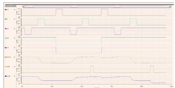
Fig. 16. Computation of NAND with 00 and 11 input combinations using 7T SRAM cells
