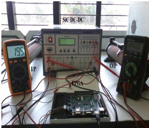
Figure 20. Input and Output voltage of step up boost converter using MPPT.
