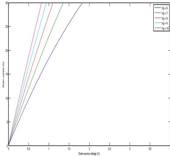
Figure 4: Output characteristics of SiC MOSFET at 150 C
