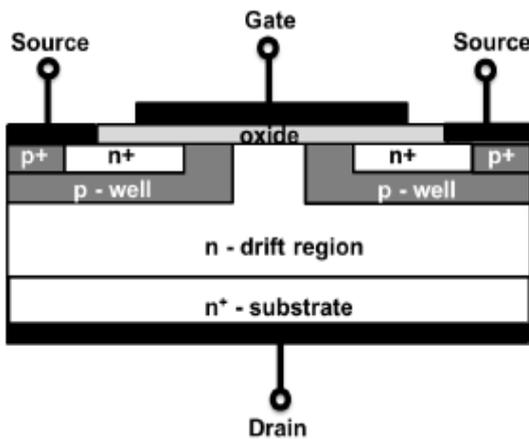
Figure 1 SiC MOSFET structure
