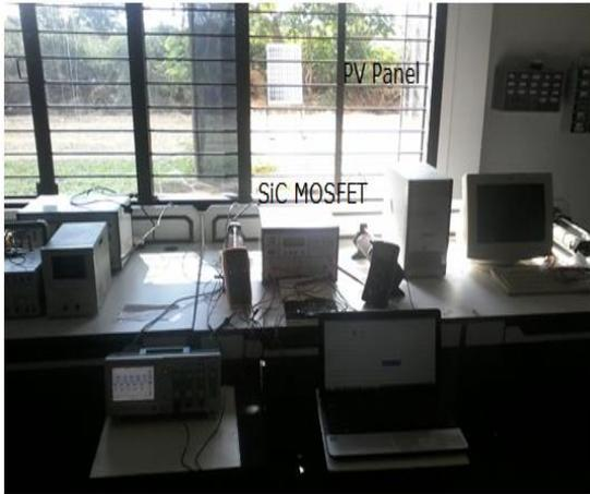
Figure.15. Hardware set-up for IC based MPPT control based photovoltaic power generation system
