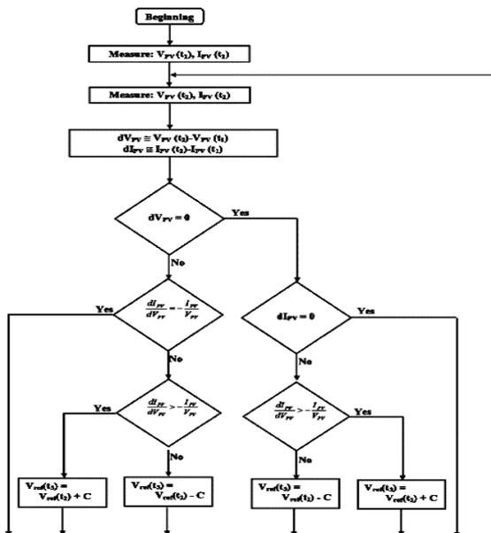
Figure 8: Flowchart of Incremental conductance method
