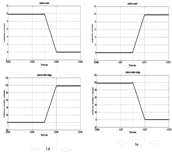
Figure .7 Determination of turn-on and turn-off time
