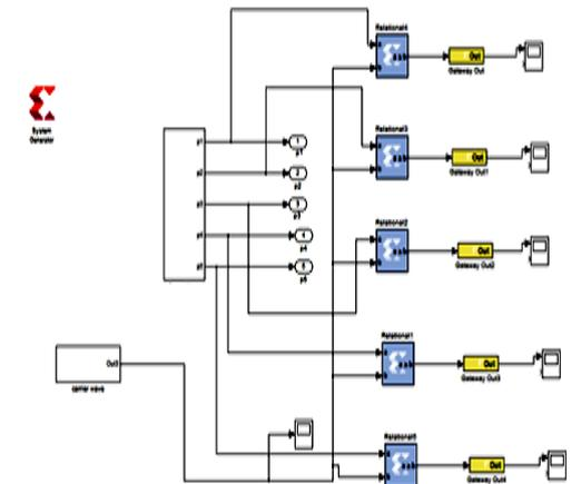
Figure 18: The logic circuit diagram in Xilinx software for the MPPT.
