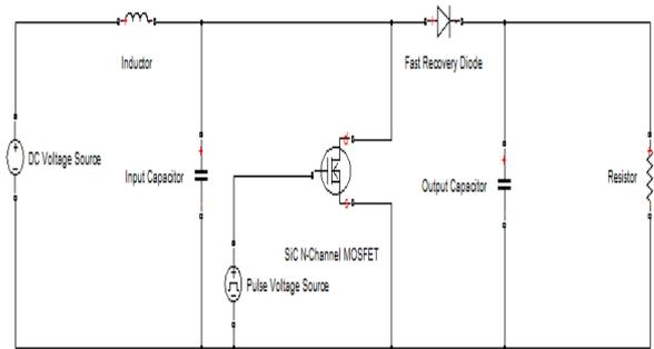
Figure 9: Circuit diagram of boost converter
