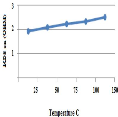
Figure 5:  $R_{DS}$  characteristic of Si MOSFET
