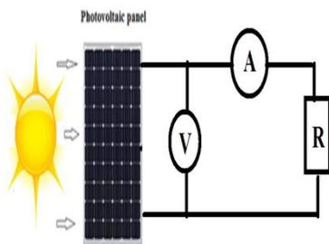
Figure 16. Experimental setup on photovoltaic panel
