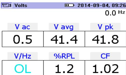
Figure 21. Output voltage ripple of SiC DC-DC boost converter for 50% duty cycle.
