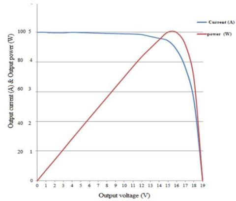
Figure 17: P-V & V-I characteristics of a photovoltaic panel
