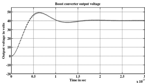
Figure .12: Output voltage of boost converter.
