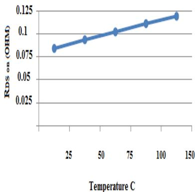
Figure 6:  $R_{DS}$  characteristic of SiC MOSFET
