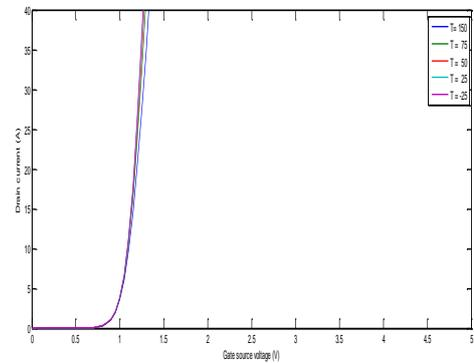
Figure 2: Transfer Characteristics of SiC MOSFET
