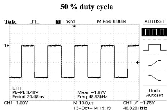
Figure.19. The change in the duty cycle of the PWM output
