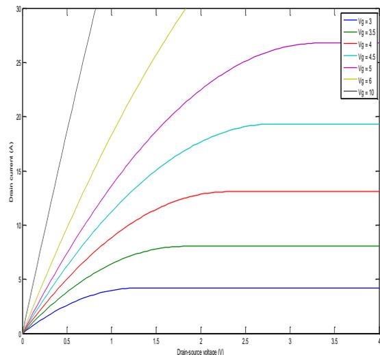
Figure 3: Output characteristics of SiC MOSFET at 25 C
