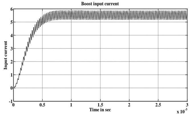
Figure .13: Input current of boost converter.
