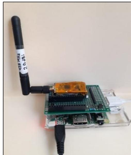
Fig 6. Raspberry Pi with the transceiver
