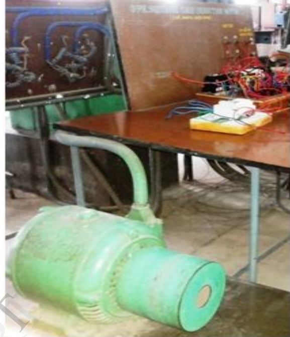
Figure 3. Connection of PLC with induction motor
