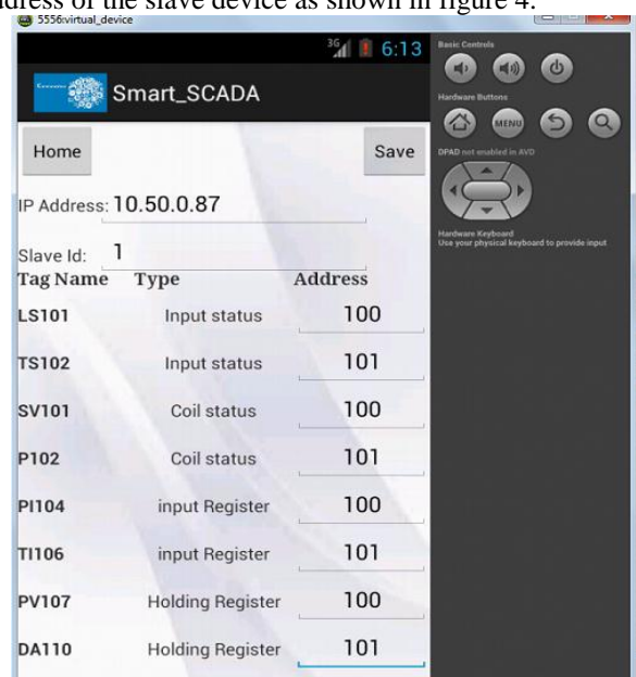
Figure.4 – Smart SCADA configuration settings
