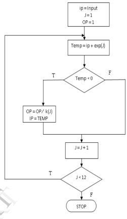
Here in each iteration, we subtract the input from the nearest value of exp(k) as listed in the table. If the difference is positive, we divide the output by the corresponding exp(k). The process continues withmore entities in our table of k, finally we get the result.
