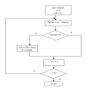
Here in each iteration, we subtract the input from the nearest value of exp(k) as listed in the table. If the difference is negative, we multiply the output by the corresponding exp(k). The process continues withmore entities in our table of k, finally we get the result. In the same way the flow chart is mentioned for nagative powers of x.
