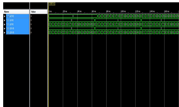
Fig. 6 Output waveform of karatsuba multiplier
