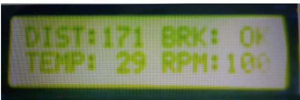
Fig. 4. Display of Distance, brake status , temperature and speed on LCD
