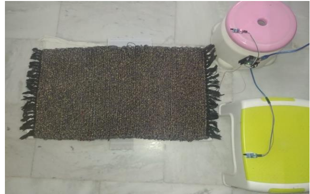
Fig. 4 Hardware of the project which includes IR sensors and piezoelectric mat
