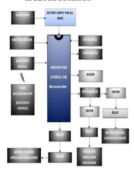
Input is given in the form of battery in volts from solar panel . vibration sensor is used for fall detection As our project contain voice recognition , bluetooth module begin used the. Controller used here Arduino the mechanical setup wheelchair is made up with motors fixed in two legs backposition when the power supplied in the patient is lifted 30 if there is any problem the buzzer indicate and its send through GSM/GPS module.
