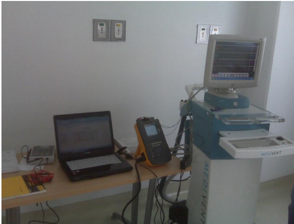
Fig 14. Electrical safety test (circuit implementation).
