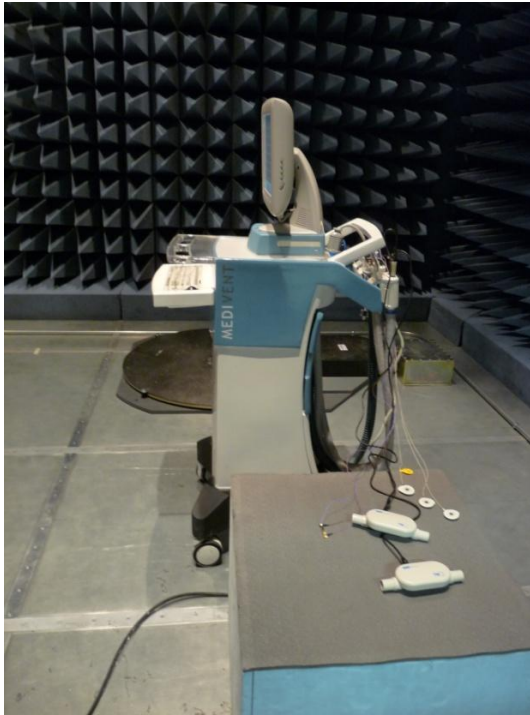
Fig. 15. Placement of the MediVent equipment and its sensors on the ground plane of the anechoic chamber
